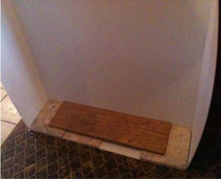
8. Lay box on its end, apply glue, lay in a 4 ft x 1 ft end section (trimmed if necessary to fit smoothly,) apply weights, let it set for a couple hours
